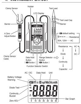
Clamp Sensor: Pick up current flowing through the conductor. Barrier: It is a part providing protection against electrical shock and ensuring the minimum required air and creepage distances
