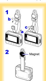
1 Attach the Z5004 to the strap/stand attachment hole.
