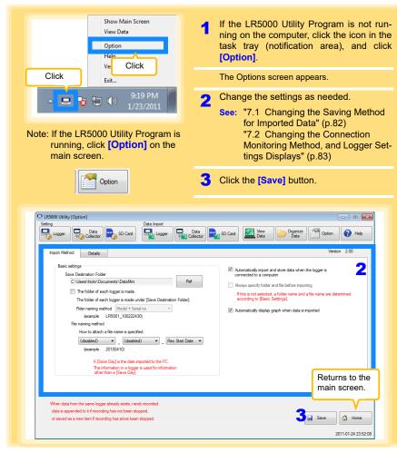
Select the [Automatically import and store data when the logger is connected to a computer] checkbox and clear the [Always specify folder and file before importing] check box to display the Data Import screen (p.60).
