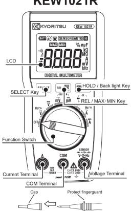
Protective figerguard: It is a part providing protection against electrical shock and ensuring the nimum required air and creepage distances.
