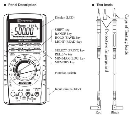
With: 1000V10A CAT. III/600V 10A CAT. IV Without: 1000V10A CAT. II/600V 10A CAT. II
