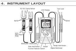
Barrier : It is a part providing protection against electrical shock and ensuring the minimum required air and creepage distances. Test Lead Cap : Test leads can be used under the CAT.II and III environments by attaching a Protective cap as illustrated below. Use of our Protective cap offers different lengths suitable for the test environments.
