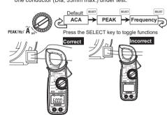
Measurement accuracy is guaranteed when the measured object is placed at the center of the Current Sensor.
