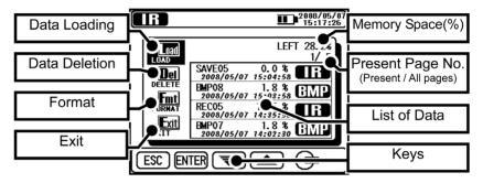
Functions to recall ( $\Rightarrow$ displays the saved data), delete ( $\Rightarrow$ deletes the saved data) and format the data ( $\Rightarrow$ formats the internal memory) are available. Details of each parameter are as follows.
