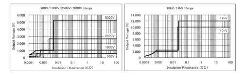
Rated current at 500V, 1000V, 2500V, 5000V Ranges : max 1mA or higher Rated current at 10kV, 12kV Ranges : max 0.5mA
