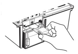
⑤ Pull up the Battery Connectors upward as indicated by arrow mark in the below left illustration, and remove them.
