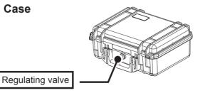
Regulating valve is to balance the air pressure in the Case hermetically sealed and external atmosphere for easy opening/closing of Case lid. Do not force to turn it or remove it.
