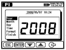
Select " I Clock Setting on the ENTER Menu (=>P.37). Adjust the time in a following order: [year], [month], [day], [hour], [minute] and [display format]. Pressing the ENTER Key confirms the entry and proceeds to next step. Press the ESC Key to return to the previous item.
