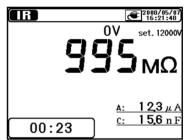
① This instrument has an auto-discharge function. With the test leads connected to the circuit under test, release the Test button to discharge capacitance in the circuit after test.
