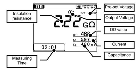
The result of DD measurement is displayed as follows.
