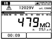
(9) Release the Button to stop the measurement. Then the measured results will be displayed on the LCD.
