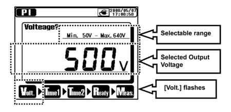
The table below shows the selectable range of voltages and step values at each Measurement Range.
