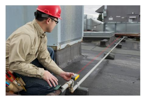
Fluke 419D Fluke 419D Laser Distance Meter
