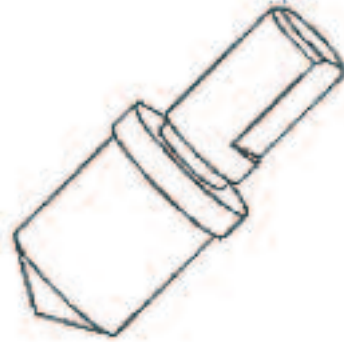
Fig.2: Diamond cone indenter
